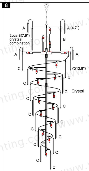
Hang crystal A on the outer frame of thebig/small lamp body. Hang crystal B on theinner ring of the small lamp body. Hangerystal C on the spiral strip.
