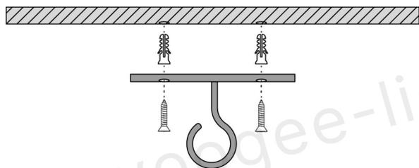
Install hook on the ceiling by using expansion screws.
