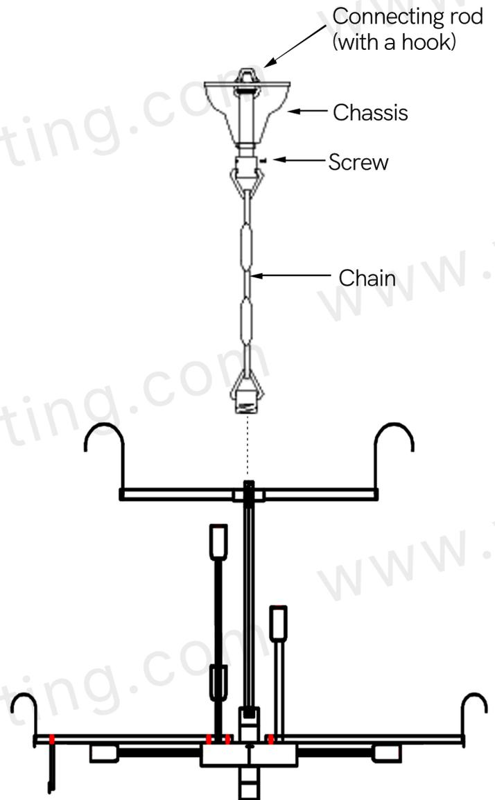
Connect the chassis to the chain via a connecting rod (with a hook), tighten the screws. Then install the chain on the lamp body.
