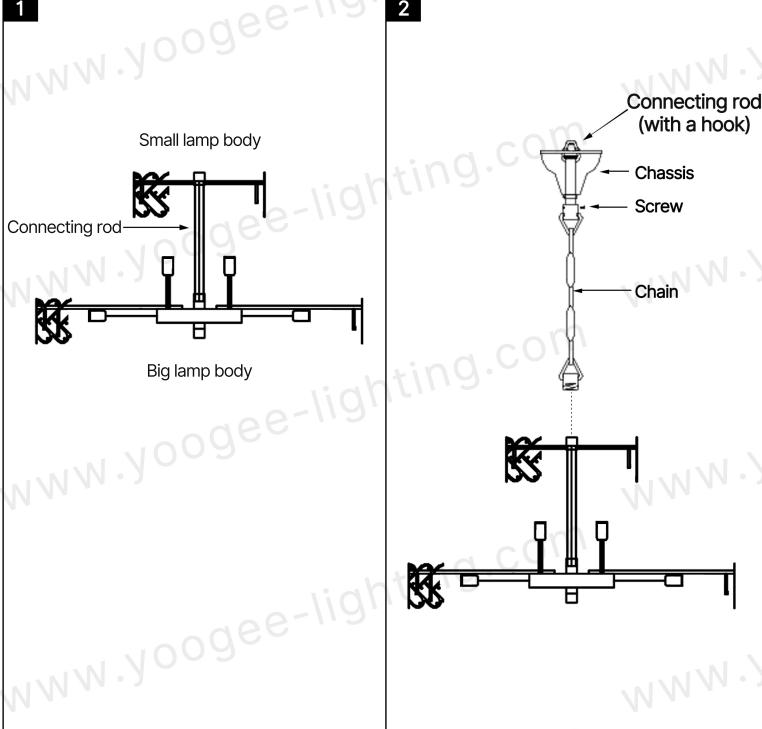
Connect the big lamp body and the small lamp body through the connecting rod. NWW.yoogee
